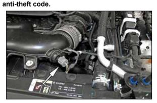
2. Disconnect the inlet air temperature sensor electrical connection and unhook the wiring harness from the intake tube.
