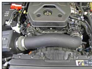
21. Install the AIRAID® intake tube into the coupler at the air filter housing and then the coupler at the throttle body and secure with the provided hose clamp
