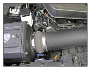
22. Connect the CCV lines to the ejection fitting installed into the intake tube.
