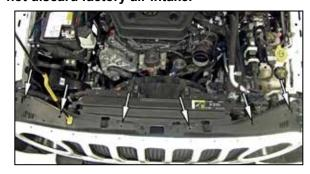
6. Remove the six retaining clips that secure the grill assembly to the core support.
