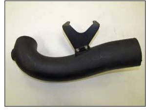
18. Install the tube mounting bracket onto the intake tube using the provided hardware.
