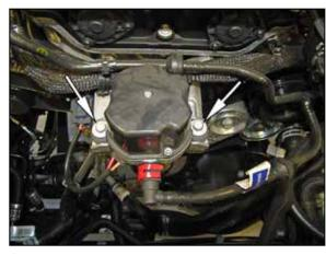
17. Remove the two bolts that secure the EVAP pump to the mounting bracket. These bolts will be reused in a later step.
